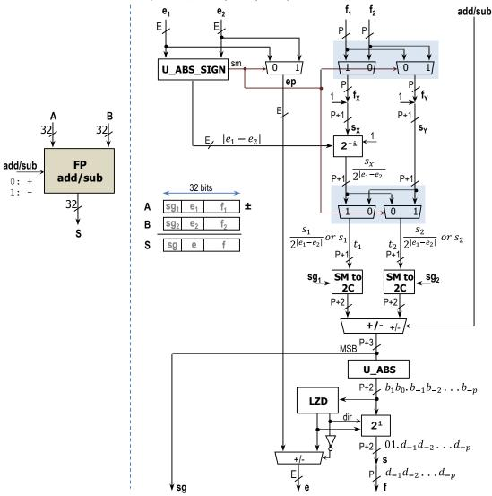
• **U\_ABS\_SIGN**: This circuit computes the absolute value of the difference of two unsigned numbers ( $e_1$  and  $e_2$ ). It also generates the signal sm.
